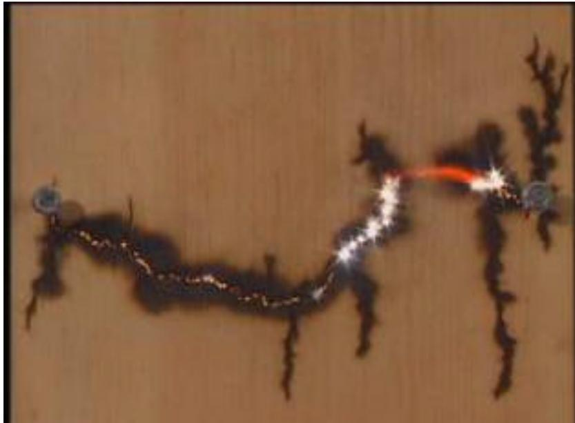
*Close-up photo of active partial insulation failure due to tracking. This type of partial failure can occur anywhere within switchgear, transformer or cable insulation and will continue until complete failure occurs. Fortunately, a new technology known as partial discharge (PD) testing, can be used to detect these partial failures so that repairs can be conducted before it's too late. PD testing is performed while your electrical system remains in service, so it doesn't interrupt operations.*
