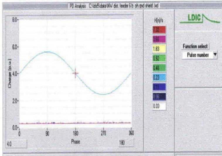
*This photo shows the results of PD testing of good insulation.*
